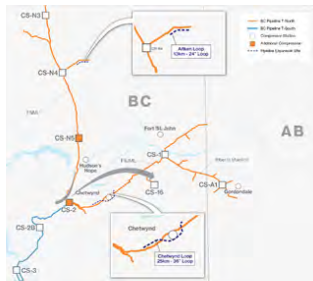
Figure 22: Spruce Ridge Extension pipeline loop extensions.
